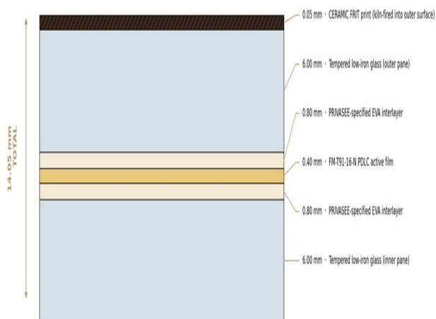
Engineering cross-section - proportional - all dimensions in mm - PRIVASEE® Smart Glass Systems
