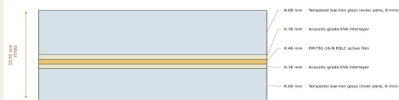
Engineering cross-section - proportional - all dimensions in mm - PRIVASEE® Smart Glass Systems
